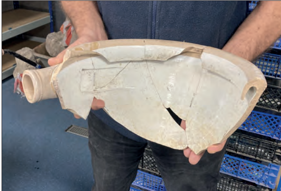
Figure 20: Part of a late 19th-century 'servant's basin' type water closet
