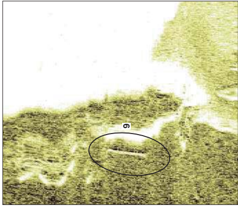
D. Waterfall image of Feature 9, linear debris (3.3m x 0.2m x 0.1m)
